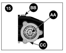
5. For AAA<sup>™</sup> pumps, refill using SIMPSON<sup>®</sup> Premium Pump Crankcase Oil. If this oil is not available, an SAE 15W-40 oil may be used.
