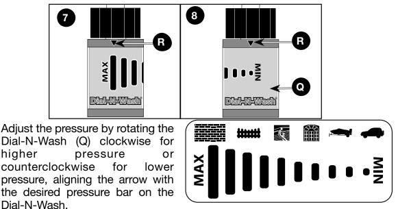
**NOTE:** To apply chemicals the black low pressure nozzle must be installed and the Dial-N-Wash must be in the MAX pressure setting.
